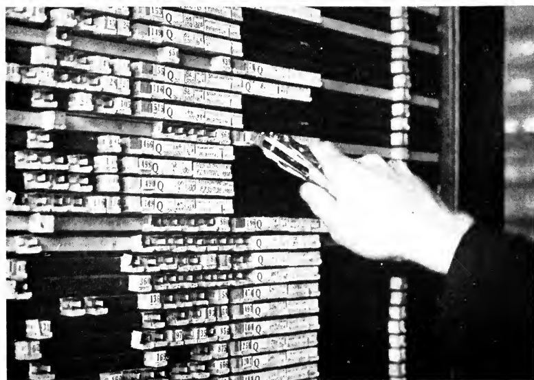
Manufacturing to stock is regulated automatically by highly organized control boards at the Franklin Automobile Company's plant. Each horizontal half-inch represents a working day. Block symbols (below) and a movable tape (left, above), schedule every operation. The boards are photographed for permanent records, and the prints are accepted as inventory statements of work in process
